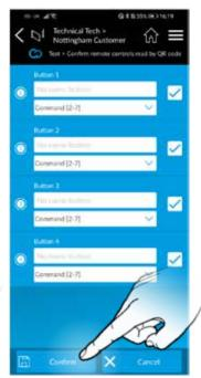
Once the QR code has been scanned, enter a Name and select the correct function for each button on the fob. If you wish for a certain button to not be active, then untick the check box for that button. Select Confirm. Repeat this process for all fobs.
