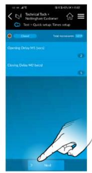
Set the Opening Delay M1 and Closing Delay M2 to the desired value (secs). Select Next.
