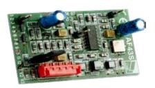
Radio frequency control card 433.92MHz
