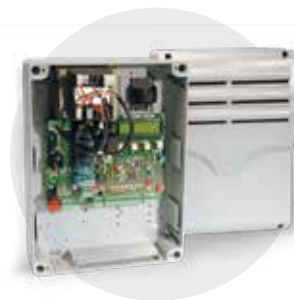
ZM3E Control Panel
