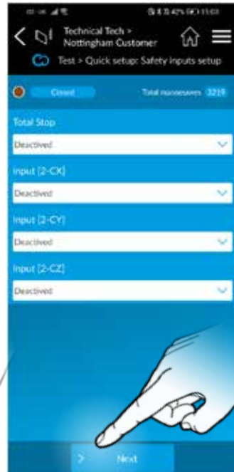
Set the safety inputs (please refer to section 12 for options). Select Next.
