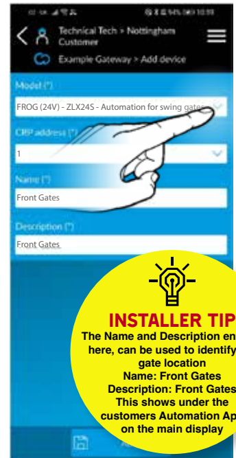
Select FROG (24V) - ZLX245 from the drop-down list. Enter a name and description, then press Add.
