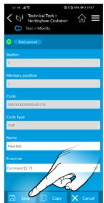
Once it has been accepted on the control panel It will display the above screen. Enter a Name and select the correct function for the fob. Select Save. Repeat this process for all fobs.
