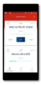
You can open, close or stop a U-link device remotely or locally with just a touch
