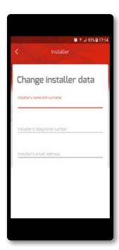
You can enter the name and references of your installer in the U-control app. In case of a system failure, the installer can be contacted directly from the U-control app, emailing also the last error detected by the central unit
