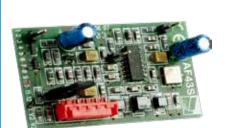
Radio frequency control card 433.92MHz
