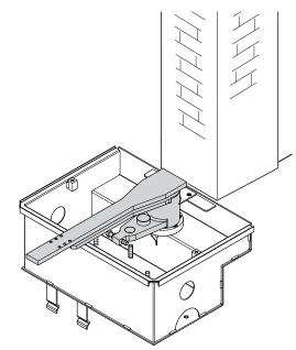
Install the gate leaf, inserting the upper hinge. Fix or carefully weld the leaf to the fixing bracket to the gate. Check that the leaf opens and closes without difficulty.
