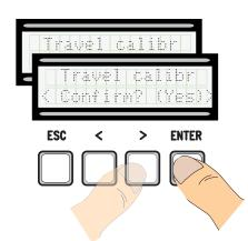
3. M1's gate leaf will perform a new closing until it completely stops...
