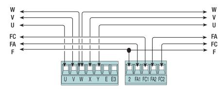
M2 - 230 V AC gearmotor with delayed closing.
