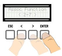
4. ... a code to enter will be requested. Send the code from the transmitter, with the swipe card or transponder.
