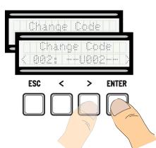
3. ... a code to enter will be requested. Send the code from the transmitter, with the swipe card or transponder.
