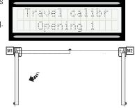
7. Once the procedure is completed, the display will read [Travel calibr OK] for a few seconds.
