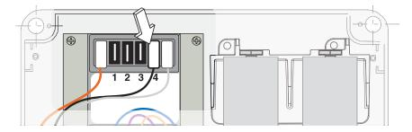
△ Before fitting any snap-in cards (such as the AF or R700), YOU MUST CUT OFF THE POWER MAINS, and disconnect the power mains.
