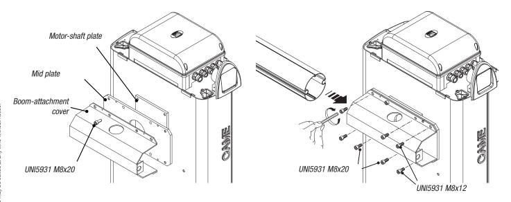
Cut the groove covering profiles to measure and fit them into either side. Use the screws to fasten the boom endcap.
