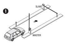
Approach the SLAVE barrier. It will automatically open only after the MASTER barrier automatically closes. The automatic closing of the MASTER barrier is excluded in the event that the safety devices detect an obstruction (such as when a car has yet to clear the MASTER barrier).
