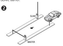
Approach the MASTER barrier. It will automatically open only after the SALVE barrier automatically closes. The automatic closing of the SLAVE barrier is excluded in the event that the safety devices detect an obstruction (such as when a car has yet to clear the SLAVE barrier).
