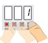
3. ... an available number between 1 and 25 will flash for a few seconds. This number is then assigned to the user after having sent the code with the transmitter or other control device (sensor, card reader or keypad selector).
