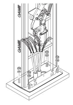
Assemble the boom-attaching cover, the mid plate and motor-shaft plate with a screw. Leave the screw loose to then facilitate fitting the boom. Fit the boom into the boom-attachment cover and fasten it using the screws.
