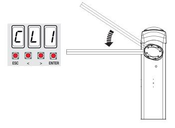
$4.\ \dots$  then, the barrier will perform an opening maneuver until the endstop point.
