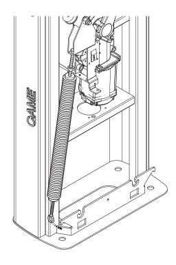
Release the gearmotor and manually turn the spring to increase or decrease tautness. The spring should stabilize at 45°. Fasten the counter nut and lock the gearmotor again.
