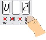
2. Select the user number to delete by using the arrow keys. Press ENTER to confirm...
