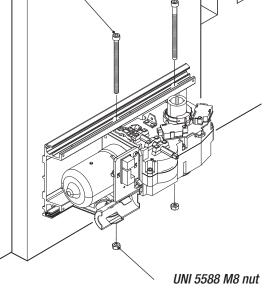
Secure the gearmotor with screws and nuts.
