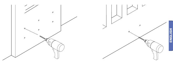
Insert the dowel or use other inserts suitable for the bracket resistance.
