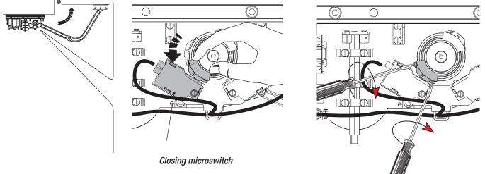
Fully open the gate-leaf of the left gearmotor and rotate the cam counter-clockwise until the closing microswitch inserts. Fix the cam with the screws.
