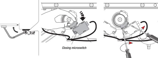
Fully open the gate-leaf and rotate the other cam counter-clockwise until the opening microswitch inserts. Fix the cam with the screws.
