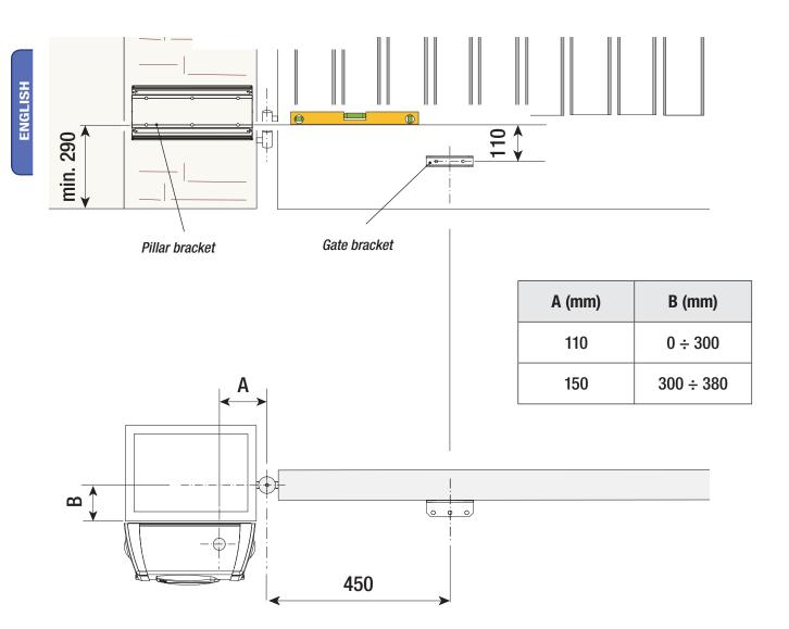
Mark the fixing points for both the pillar and gate brackets, respecting dimensions indicated in the drawing.
