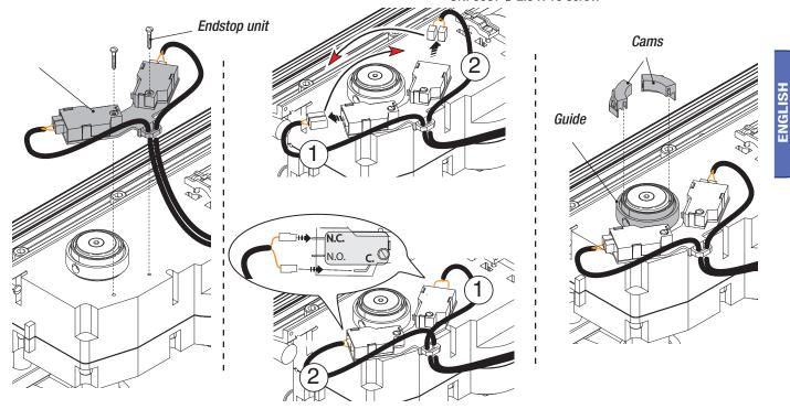
Fully close the gate-leaf of the left gearmotor and rotate the cam clockwise until the closing microswitch inserts. Fix the cam with the screws.
