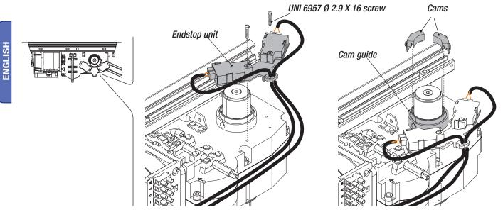
Fully close the gate-leaf of the left gearmotor and rotate the cam counter-clockwise until the closing microswitch inserts. Fix the cam with the screws.
