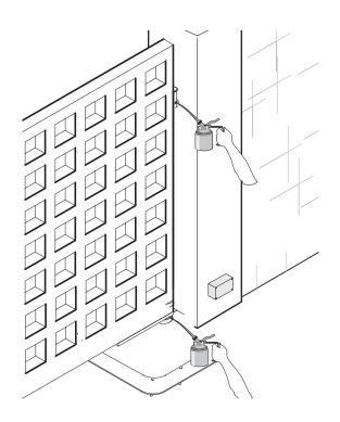
Make sure there are no plants within the photocell's beam, and that the gate motion is free of any obstacles.
