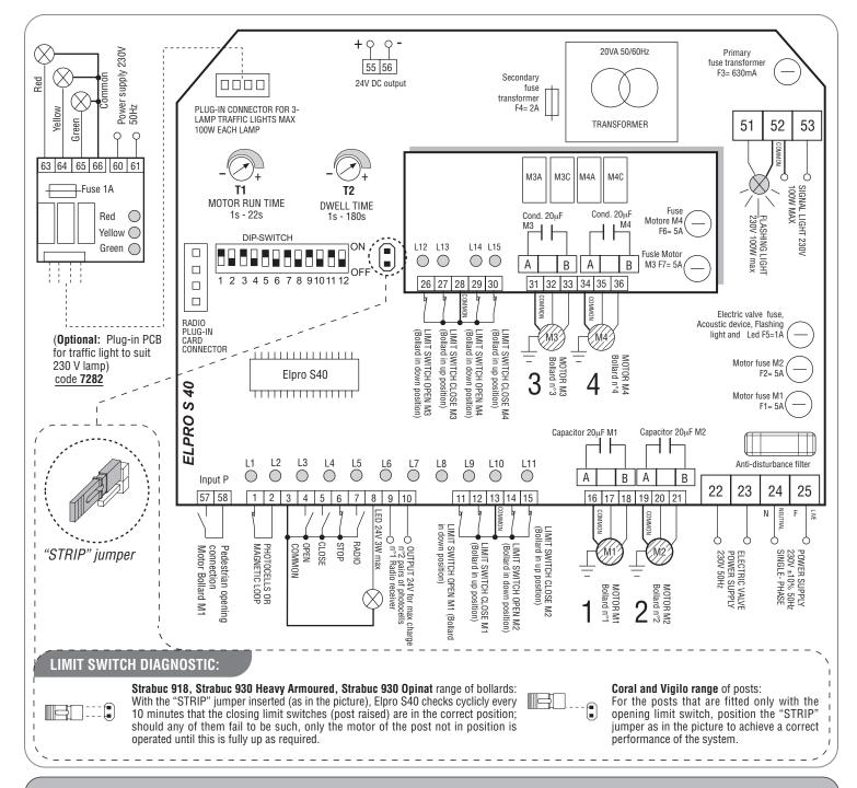
Note well: Whenever Elpro \$40 is re-powered, wait 10 seconds for the logic to become fully operating again.
