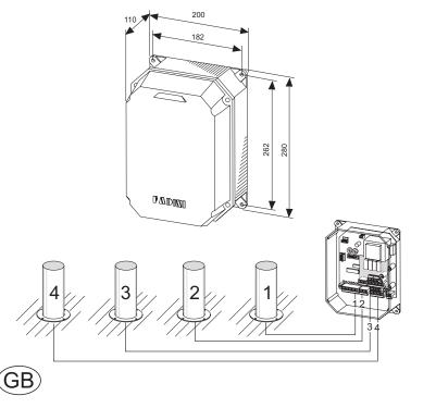
Elpro S40 is a control panel fitted with microprocessor, specially designed to operate the Strabuc, Coral and Vigilo range of electro-hydraulic bollards. Its main feature is the option to be able to control up to 4 bollards at the same time.
