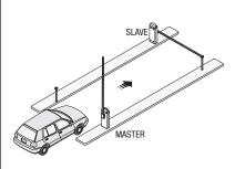
Approach the SLAVE barrier which will open automatically only after the MASTER barrier has closed automatically.
