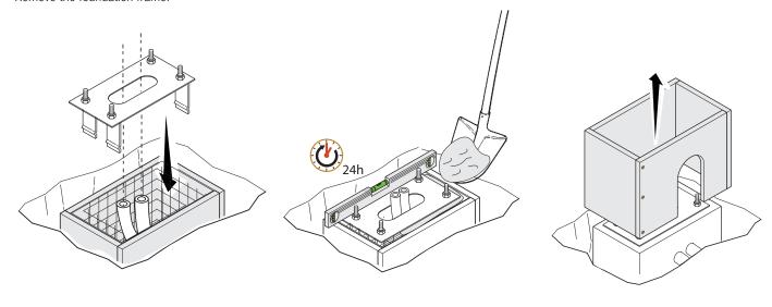
Fill the hole with earth around the concrete block.
