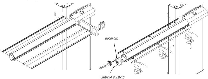
Place the anti-shearing protective cover over the boom-attachment cover and fasten it in place using the screws.
