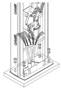
Assemble the boom-attachment cover, intermediate plate and the motor shaft plate with a screw. Leave the screw loose to make it easier to insert the boom.
