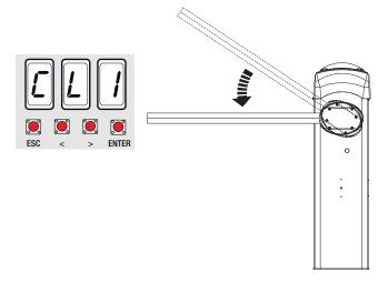
4. ...then the operator opens until it reaches the limit-switch point.
