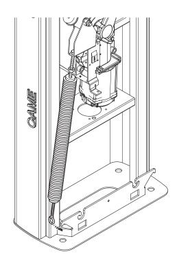
Release the gearmotor and manually turn the spring to increase or reduce the traction. The boom should stabilise at 45°. Fix the counter nut and lock the gearmotor again.
