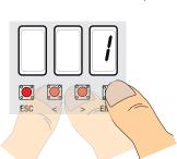
3. ... an available number between 1 and 25 flashes for a few seconds. This number is assigned to the user after the code has been sent from the transmitter or another control device (sensor, card reader or keypad selector).
