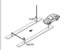
Approach the MASTER barrier which will open automatically only after the SLAVE barrier has closed automatically.
