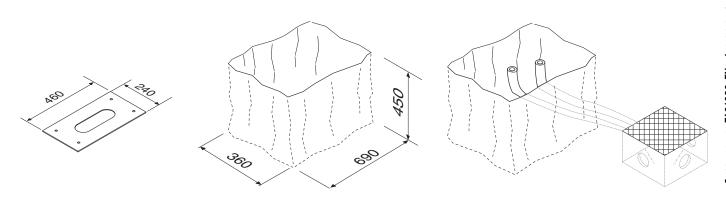
Prepare a foundation frame that is larger than the anchoring plate and sink it into the dug hole. Insert an iron cage into the foundation frame to reinforce the concrete. Attach the four anchoring clamps to the anchoring plate.
