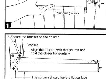
1. From the centre pivot line of the hinges, measure 222mm(8-3/4")
