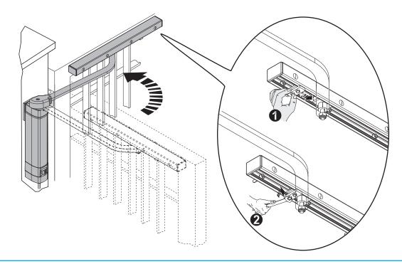
**6** - Open the lower cap and make the necessary electrical connections; - Close the lower cap again..
