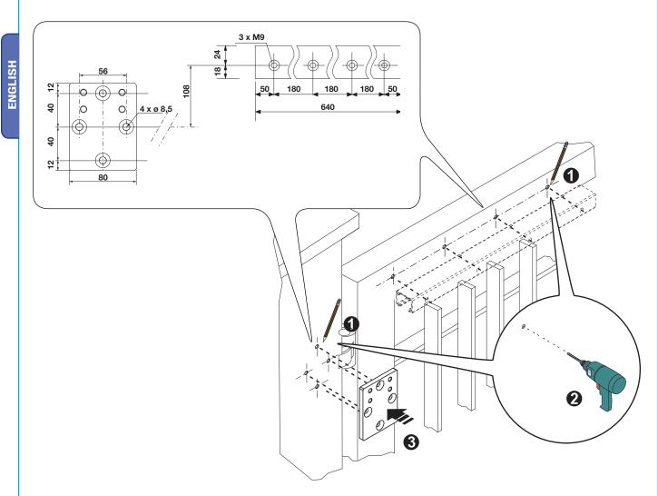
Drill and thread the holes using an M8 male piece or use  $\emptyset$  11 mm threaded inserts or any suitable materials for the rail to hold. Note: the illustrations are mere examples, it is up to the installer to choose the most suitable solution depending on gate-leaf type and thickness.
