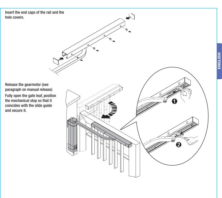
Fully close the gate leaf and position the closing mechanical stop so that it coincides with the slide guide and then secure it.
