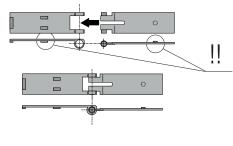
4) Insert the hinges into the box (either on the right or left side, as you prefer) and secure them using the supplied nuts and bolts.
