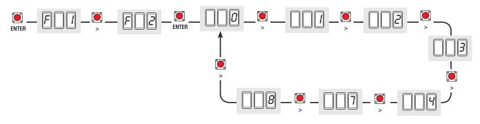
**F 3 (CY Input):** safety contact input can take on the following functions: C1 (re-opening when closing), C2 (re-closing when opening), C3 (partial stop), C4 (obstacle stall), C7 (re-opening when closing, for sensitive edges), C8 (re-closing when opening, for sensitive edges) or, be deactivated.
