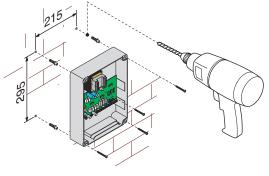
2) Perforate the pre-punched holes and insert the cable glands with the corrugated tubing for the electrical cables to travel through.
