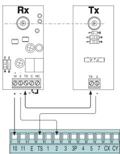
At each opening and closing command, the control board assesses the efficiency status of the safety devices (photocells). Any anomaly found is signaled with the flashing of the LED on the control board. Consequently it cancels any commands coming from the transmitter or the button.
