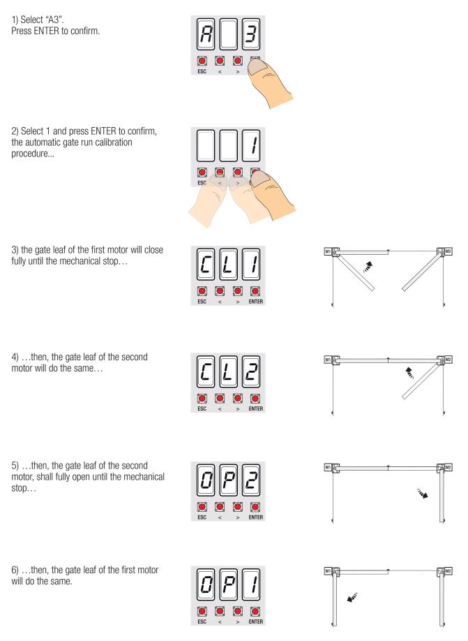
Note: the slow-down areas and points at which the gate draws to the fully open or closed position are tested according to the parameters set forth by Technical Norms EN12445 and EN12453 regarding compatibility of impact forces generated by moving gate leaves.
