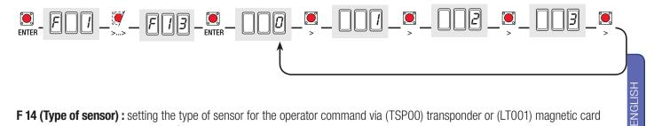
F 14 (Type of sensor) : setting the type of sensor for the operator command via (TSP00) transponder or (LT001) magnetic card reader with R700 encoder card or S7000 keyboard with R800 encoder card.
