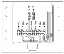
Connect the controller MO 90 with the junction box in the motor lock like followed (see also chapter 7.).
