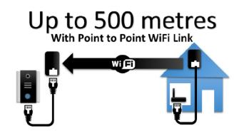
Range can be extended up to 500 metres by using various open market devices, such as Homeplug Technology, WiFi repeaters and point to point links. Always conduct a site survey before quoting this system.
