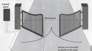
Exit sensor between 5m and 18m from the gate
