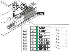
Connect the devices to terminal board CN9.
