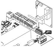
The quick insertion connector JP1 is specifically for 5-pin FAAC radio or decoder boards.
