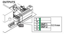
The E844 3PH has two Open Collector outputs that are activated according to programming functions of and oc.
