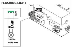
The flashing light indicates that the gate is moving and must be installed in a position that is visible from both sides of the gate.
