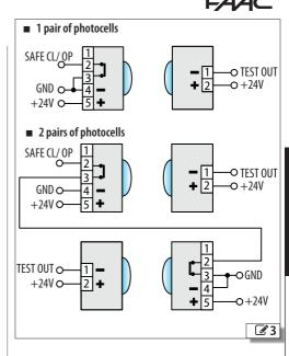
DO NOT connect photocells if the SAFE input is configured to connect a sensitive edge.
