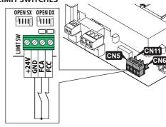
In order for to operate correctly, the E844 3PH board has to be connected to the opening and closing limit switches.
