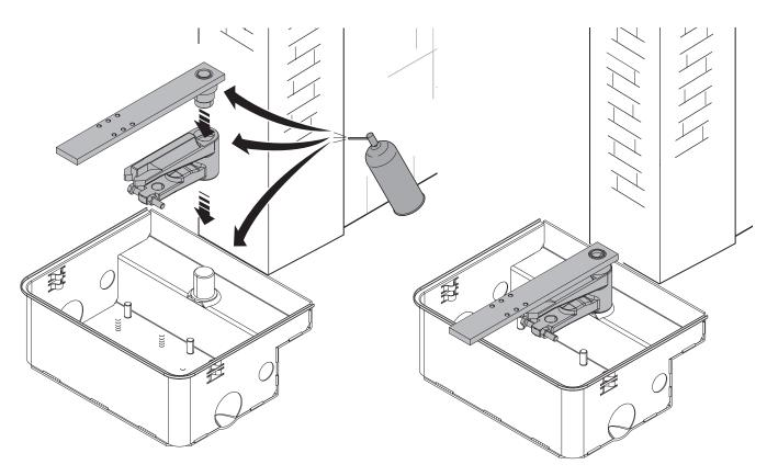
Install the gate leaf, inserting the upper hinge. Check that the leaf opens and closes without difficulty. Carefully fix or weld the door to the gate fixing bracket.
