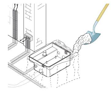
Position the box level with the ground and place the pin in line with the upper gate hinge. Wait at least 24h to cure. Clean any remaining concrete from inside the box.
