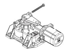
Open the leaf to simplify gearmotor installation and securing inside the foundation case.
