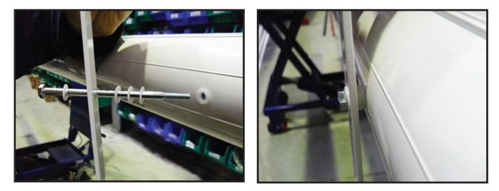
**3.** Repeat with another strip on the other side of the beam, ensure that both vertical strips are orientated with their tips bending away from each other.
