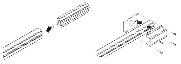
Fix the boom to the anchoring plate.
