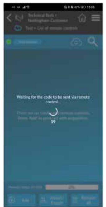
If you pressed Local Acquisition, the screen will change to the one shown here. Select the button on the fob and it will add the button straight onto the control panel.
