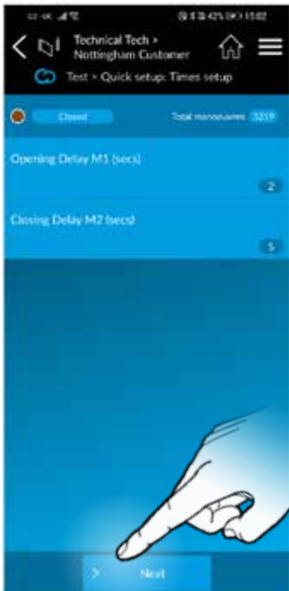
Set the Opening Delay M1 and Closing Delay M2 to the desired value (secs). Select Next.
