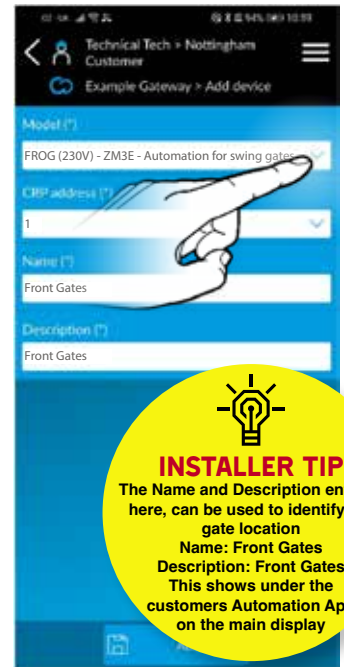
Select FROG (230V) – ZM3E from the drop-down list. Enter a name and description, then press Add.
