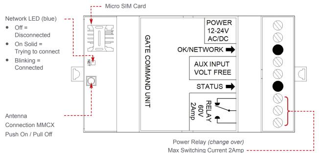
Max Switching Voltage 60V AC or DC
