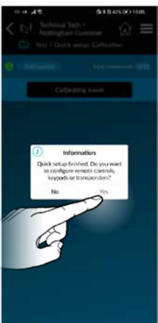
When the gate has successfully calibrated, it will automatically display the dialog box shown below. Select Yes.
