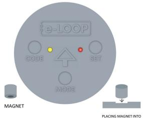
PLACING MAGNET INTO BUTTON RECESS.
