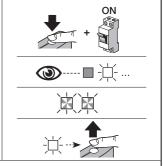
(\*3) Note - If the LED emits a steady red light, it means that the memorisation procedure was not completed. In this case, repeat the procedure from the beginning.
