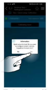
When the gate has successfully Select Add. calibrated, it will automatically display the dialog box shown below. Select Yes.
