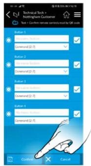
Once the QR code has been scanned, enter a Name and select the correct function for each button on the fob. If you wish for a certain button to not be active, then untick the check box for that button. Select Confirm. Repeat this process for all fobs.
