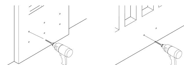
Insert the anchors or use suitable inserts for holding the brackets.
