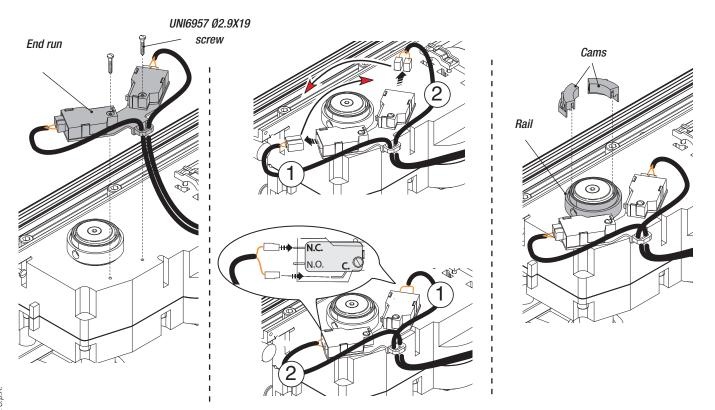
Open the leaf fully and turn the cam clockwise until the opening microswitch is activated. Secure the cam with the screws.
