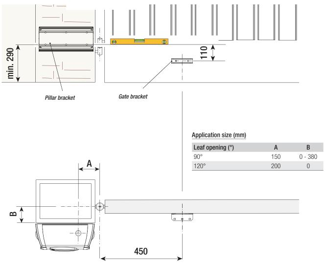
Mark the fixing points on the pillar bracket and gate bracket, respecting the values shown in the drawing.
