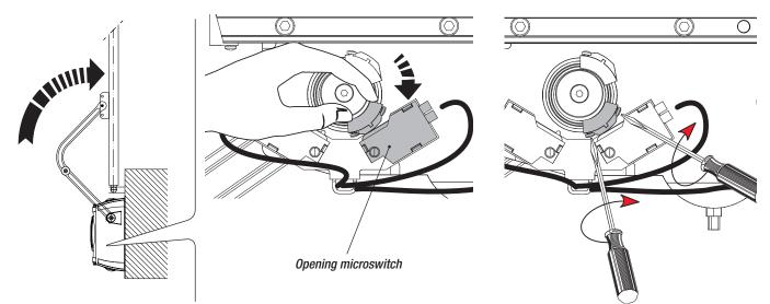
Close the leaf fully and turn the other cam anti-clockwise until the closing microswitch is activated. Secure the cam with the screws.
