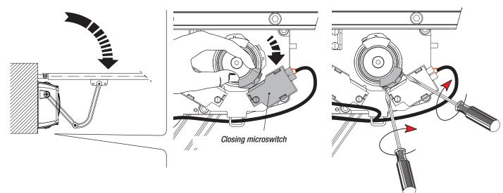
For right-hand gearmotor. Secure the end run to the gearmotor, invert the microswitch cables and insert the cams on the guide.
