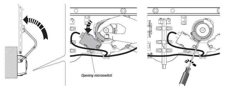
Close the leaf fully and turn the other cam clockwise until the closing microswitch is activated. Secure the cam with the screws.
