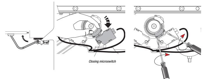
Fully open the leaf and turn the other cam anti-clockwise until the opening microswitch is activated. Secure the cam with the screws.
