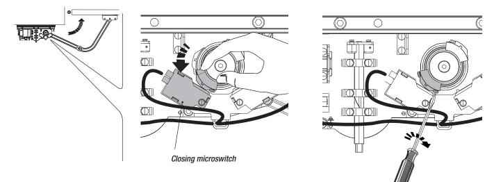
Fully open the leaf and turn the other cam clockwise until the opening microswitch is activated. Secure the cam with the screws.
