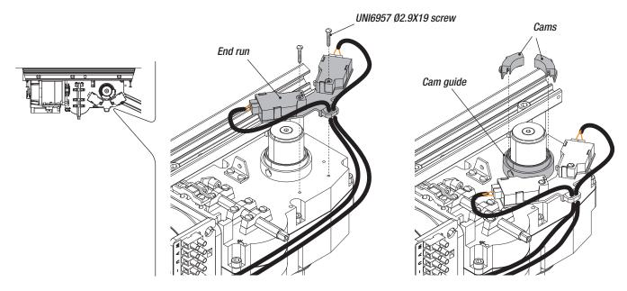
Open the leaf fully and turn the cam anti-clockwise until the opening microswitch is activated. Secure the cam with the screws.
