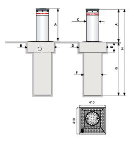
Each bollard comes with 10 metres of electric cables for motor, limit switches, solenoid valve, led lights where fitted.
