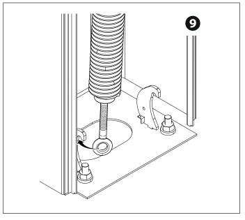
Lubricate the spring when it is fully extended.
