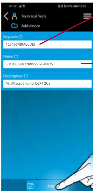
3.8 Manual Add Enter the "Keycode" located on the front of the RGSM001S. Enter a "Name" and "Description" followed by "Add".
