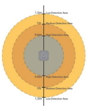
Varying magnetic eld detection zones. The grey area depicts a 0.6m high sensitivity detection area surrounding the e-loop, suitable for the majority of vehicles. The dark colour area depicts a 1m medium sensitivity detection area surrounding the e-loop, suitable for most vehicles. The light colour area depicts a 1.5m low sensitivity detection area surrounding the e-loop, which is only suitable for some vehicles.
