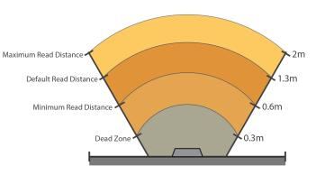
Radar detection range. Spanning from a 60° FOV from the e-loop, these are the range zones. The grey area depicts the dead zone, in which objects cannot be detected. The Minimum read distance is 0.6m. The default read distance is 1.3m, and the Maximum read distance spans up to 2m.
