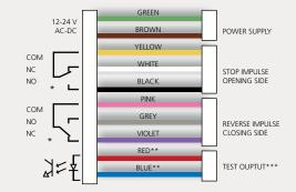
\* Output status when sensor is operational \*\* For compliance with DIN 18650, connection to door controller test output is required. \*\*\* If door controller is not tested: conncect BLUE to 0 V and RED to +12 V - 30 V DC
