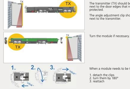
The transmitter (TX) should be placed next to the door edges that need to be protected.
