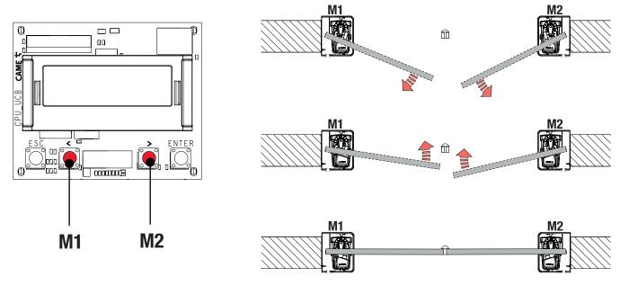
With the leaf shut, loosen the closing limit switch screw until it touches the transmission lever. Tighten the nut to lock the screw into position.
