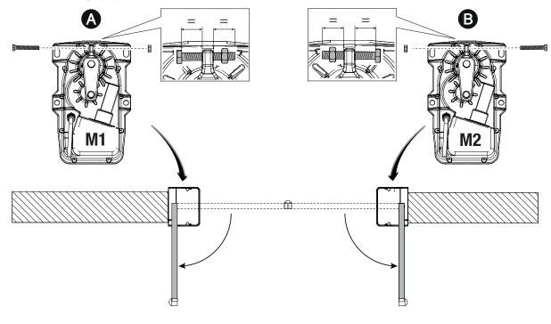
Position the gearmotor over the threaded pins of the casing and fasten it.
