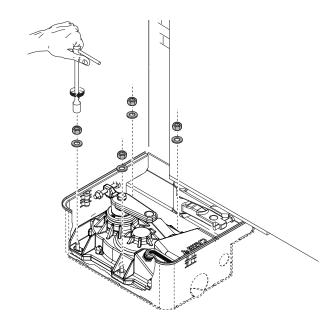
Lubricate the transmission lever.
