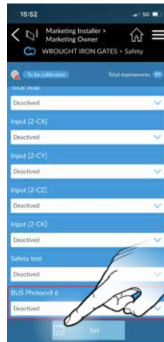
3 Each connected set of photocells will show as a different numbered device from 1 to 8 depending on the dip switch BUS address setting.
