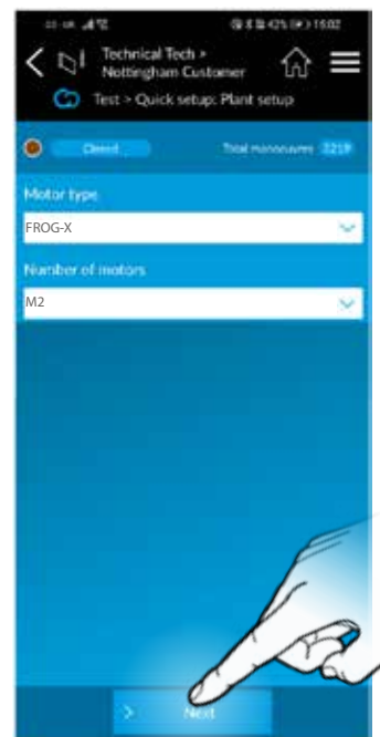
Ensure Motor Type and Number of Motors is set as above, then select Next.
