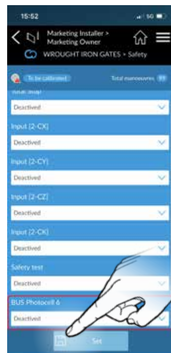
3 Each connected set of photocells will show as a different numbered device from 1 to 8 depending on the dip switch BUS address setting.
