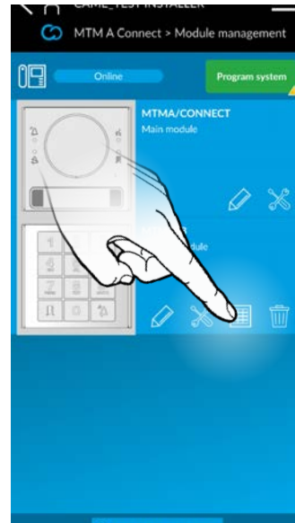
5.3 We will be asked to confirm the choice, and once done, the devices will be shown in order. Now press the PIN pad icon on the right of the keypad image to program to pin codes
