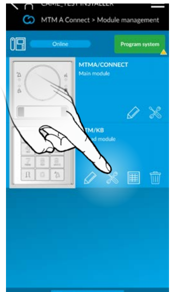
5.8 The DEFAULT operation for entering a PIN code to gain access to a property is for the user to first press the DOOR button (or the ★ button) - bottom left on keypad (depending on model of keypad fitted) – then the PIN code, followed by the DOOR or ★ button again. In order to change this so only the PIN code is required (without the need to press anything else), you must change the PIN Access Mode. Press the Tools icon as shown.
