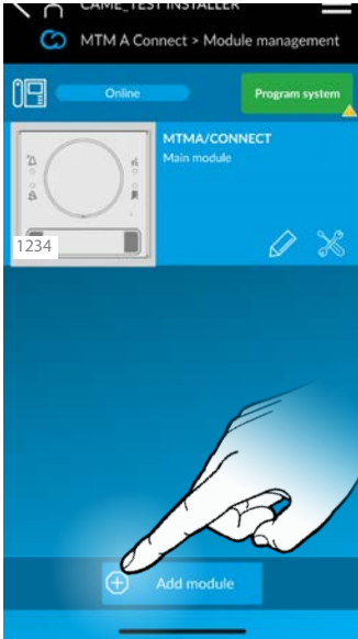
5.1 To add in an additional MTM module to the unit, we need to press “Add module” at the bottom.
