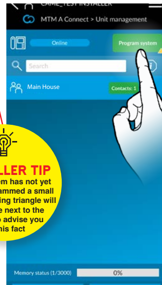
4.20 If you wish to add more contacts to the Main House, simply select it again, add another contact, and change the order required for them to be called in. When done press the GREEN Program system button on the top right.
