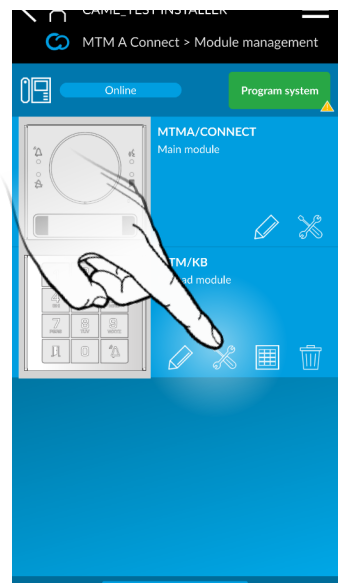
5.8 The DEFAULT operation for entering a PIN code to gain access to a property is for the user to first press the DOOR button (or the ★ button) - bottom left on keypad (depending on model of keypad fitted) – then the PIN code, followed by the DOOR or ★ button again. In order to change this so only the PIN code is required (without the need to press anything else), you must change the PIN Access Mode. Press the Tools icon as shown.
