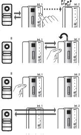
With a call active, select the internal receiver to which the call is to be transferred.
