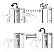
To call an internal receiver, pick up the handset and press the button for the receiver you want.
