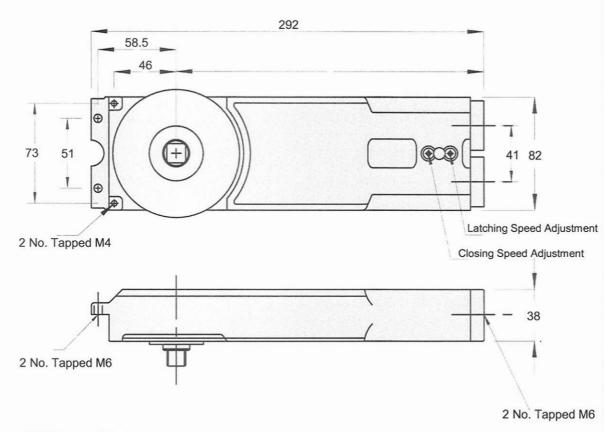
NOTE: It is important to incorporate a stop in the gate design to limit the opening to approx 90° to prevent damage to the unit.
