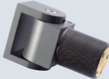
SureClose 57 W Code: 75057114m SELF-CLOSING FROM 85° • Holds gate open at 90° (not suitable for pool/safety gates) • Gate sweep: 90° in and out • Adjustment tool included
