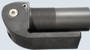
SureClose 108 AT90 W Code: 75108214m SELF-CLOSING FROM 85° • With final snap-close action • Gate sweep: 180° one way • Holds gate open at 90°–180° (not suitable for pool/safety gates) • Adjustment tool included
